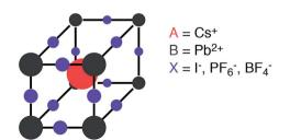
Fig. 1 Schematic of the perovskite crystal structure composed of two cations (A and B) and an anion (X). Here we consider both elemental and molecular anions.
